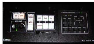
The Smart Panel controller which is used to turn the projector on is located on top of the multimedia cart.
