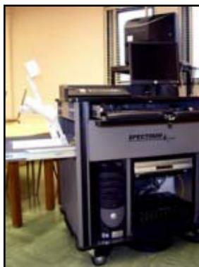
Smart Classrooms contain a “Smart Cart”, ceiling projector, and screen. The standard cart configuration is a computer with a monitor, a VCR/DVD combo, and possibly a document camera sometimes called an ELMO. The device that allows all the hardware to work together is called a controller. The controller
