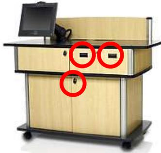
Step 2: Push button on Tower CPU to turn on Computer
