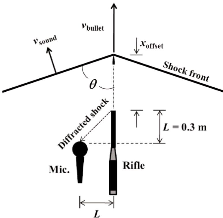
Figure 3. The supersonic bullet creates a shock cone of half-angle  $\theta$ . The apex of the cone propagates forward at the speed of the bullet. Normal to the wavefront, propagation occurs at the speed of sound. At the moment the shock front reaches the microphone (by diffraction), the bullet has advanced a distance  $x_{\text{offset}}$ .
