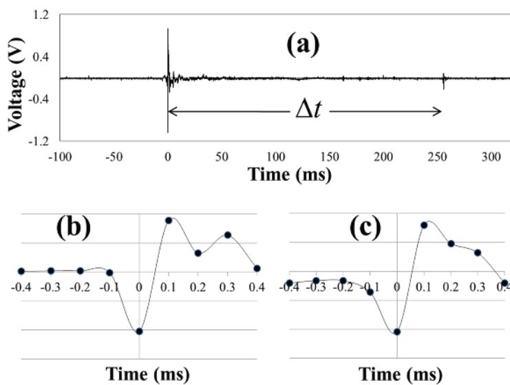
Figure 2a is a plot of voltage as a function of time obtained by downloading the microphone signal captured by the oscilloscope (for  $d = 45$  m). Compared to the large initial gunshot signal, the reflected sound is considerably attenuated but still discernable. In Figures 2b and 2c, the original and reflected signals are displayed, respectively, with amplified scales. That the two signals are very similar in shape is evidence of their common origin.
