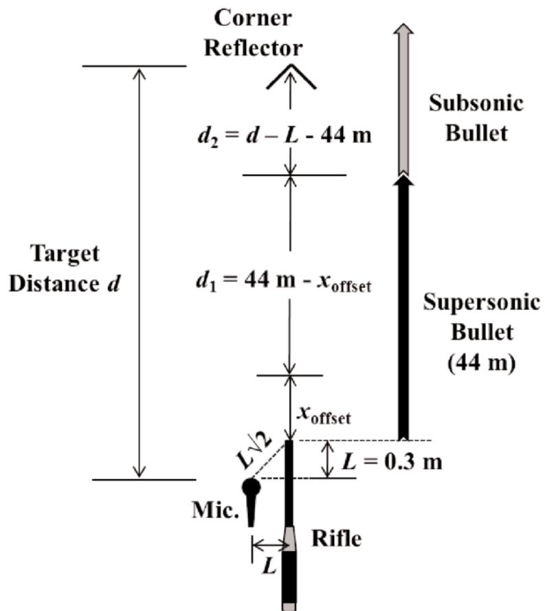
Figure 5. Accounting of the distances needed to correct the sonic data.
