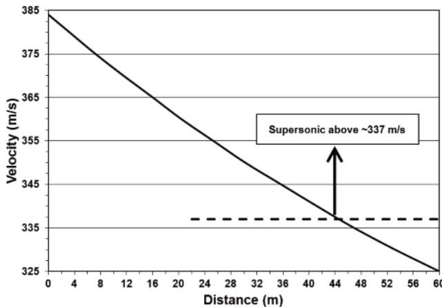
Figure 4. Velocity values for a Federal 22-caliber bullet (36-grain, model 745) at various downrange distances, obtained from commercial ballistics software. The bullet is supersonic out to a range of 44 m.
